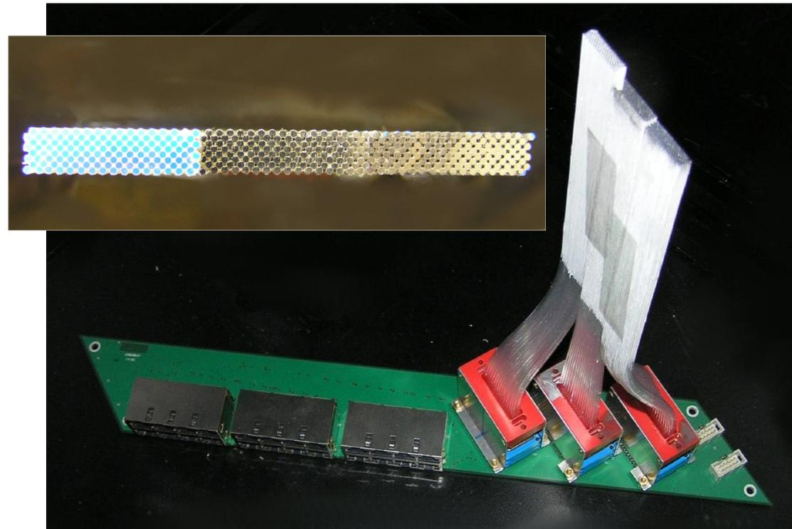
[triple detector mounted on front-end board with 96 read-out channels (384 fibres)]
