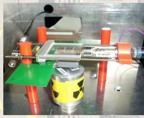
Boron disc arranged as absorber material
