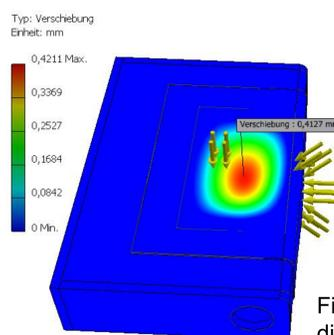
Finite element analysis of a 0.5 mm thick titan disk on an aluminium frame
