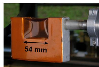
First evacuated target chamber model with a thin wall thickness in the sensor area for less  $\Xi^-$  stopping:
