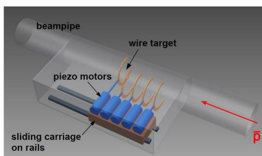
Design of a steerable and exchangeable wire target
