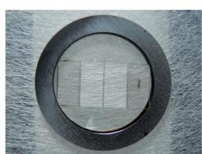
Picture of the carbon filament prototype (3  $\mu\text{m}$  x 100  $\mu\text{m}$ )
