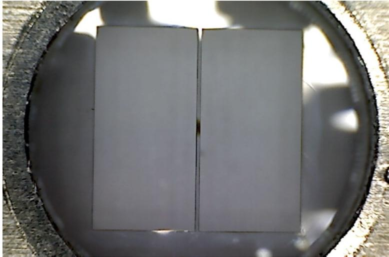
Figure 3.6: Black spot on the diamond filament after being irradiated with electrons.
