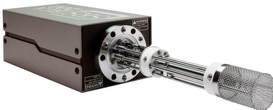
Figure 5.17: Residual Gas Analyzer RGA 200.
