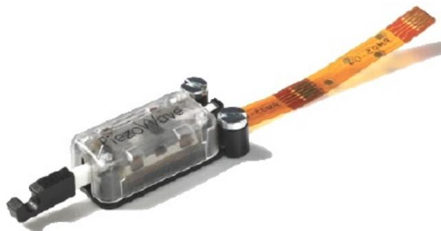
Figure 5.3: PiezoWave 0.1N motor[78].
