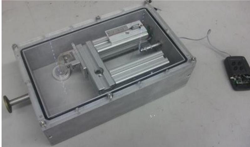
Figure 5.11: View from above of the vacuum chamber with the metal structure inside of it.
