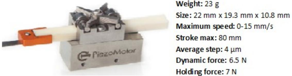
Figure 7.1: PiezoLeg motor plus the specifications provided by the manufacturer [88].
