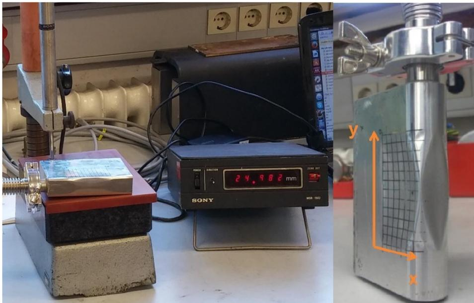
Figure 4.3: Left side: Chamber connected to the vacuum pump with the precision needle measuring its deformation. Right side: AlMg  $100\ \mu\text{m}$  rounded chamber deeply deformed when pumped.
