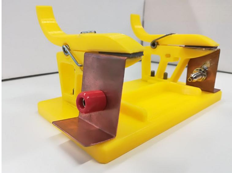
Figure 3.2.: This picture shows the holding device used throughout the experiments. It consists of a 3D-printed nonconductive frame onto which two copper plates with plugs are applied. The fiber can be pressed onto these plates allowing its inclusion into a circuit.
