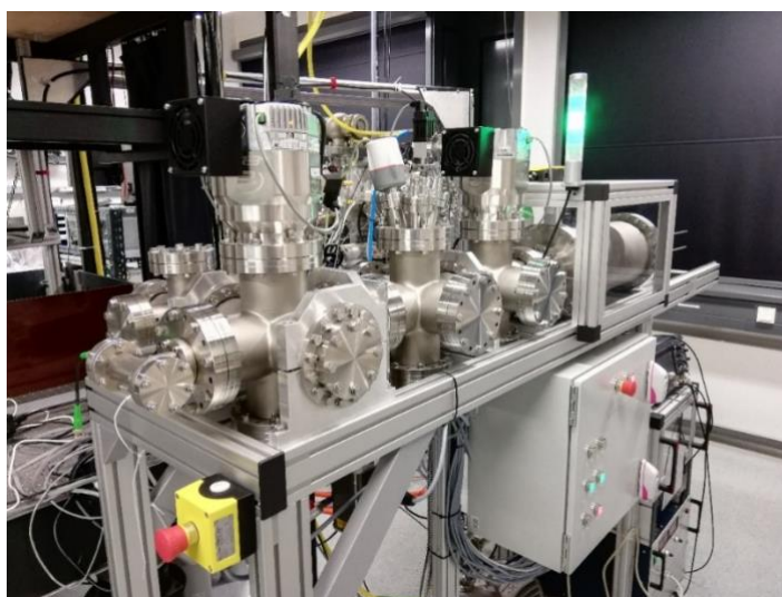
Fig. 9: Current source part of the TACTICa setup. The recoil ion source is mounted at the end of the vacuum chambersetup in the right-hand side of the photo.
